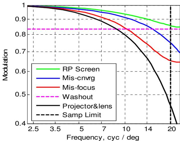
**Figure 9. The black solid curve indicates the projector MTF under optimal conditions. The remaining curves show the reductions in MTF caused by the RP screen, mis-convergence, mis-focus, and washing out the image to a contrast ratio of 10:1.**
