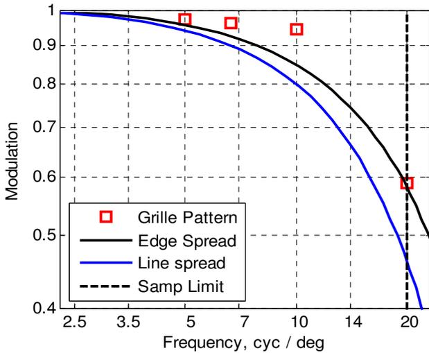
**Figure 6. Modulation Transfer Functions computed from the Edge Spread Function shown in Figure 4 and the Line Spread Function shown in Figure 5. The red boxes indicate the modulations measured at four discrete frequencies using the grille pattern method.**
