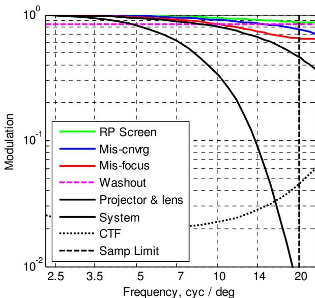
**Figure 10.** The lower black solid curve indicates the MTF of the display system with an antialiasing filter width of 1.1 pixels, bi-cubic image warping, and a well focused and converged projector on the front projection screen. The five curves shown in Figure 9 are included for comparison.
