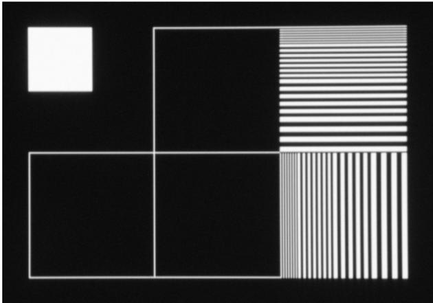
**Figure 2. Photograph of the line/grille test pattern used to measure the “continuous” system components. This pattern was generated using the same computer and software as described above.**
