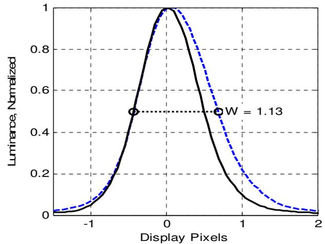
**Figure 8. Line spread functions for the mis-converged horizontal line and the well converged vertical line in the line/grille pattern shown in Figure 7.**
