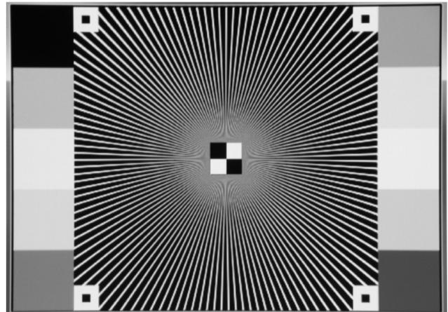
**Figure 3. Photograph of the radial grating test pattern used to measure the resolution of all components of the display system.**
