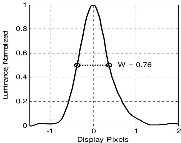
**Figure 4.** First difference of the edge spread function (ESF) for a horizontal luminance scan across the vertical edges of the white square in the upper left corner of Figure 2. The half-maximum width of this function was 0.76 pixels.
