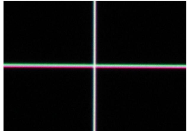
**Figure 7. Close up photograph of the line intersection from Figure 2 illustrating the distinct color mis-convergence occurring in the vertical direction.**
