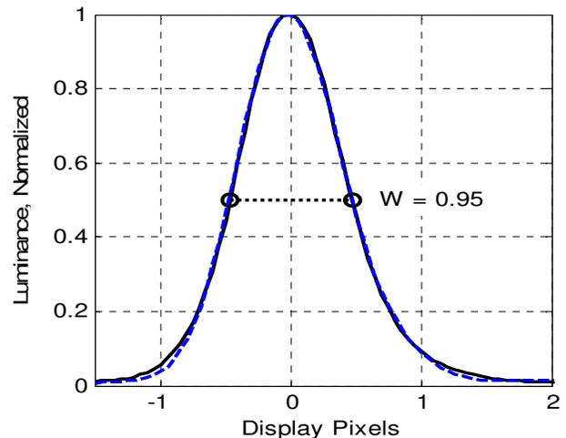
**Figure 5.** Measured line spread function (LSF) is shown as the solid black line. The dashed blue line shows the result of convolving the ESF from Figure 4 with a rectangular “pixel aperture” with a width of 0.72 pixels.
