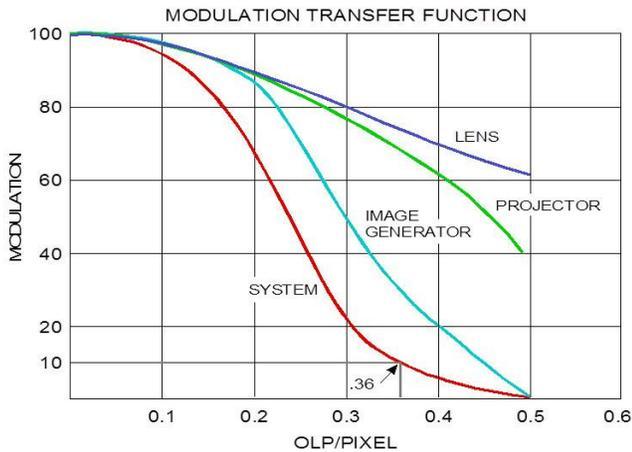
**Figure 1. Modulation transfer functions for three major system components (lens, projector, and image generator) as a function of spatial frequency. From Black (1998). Figure courtesy of P. Lyon.**
