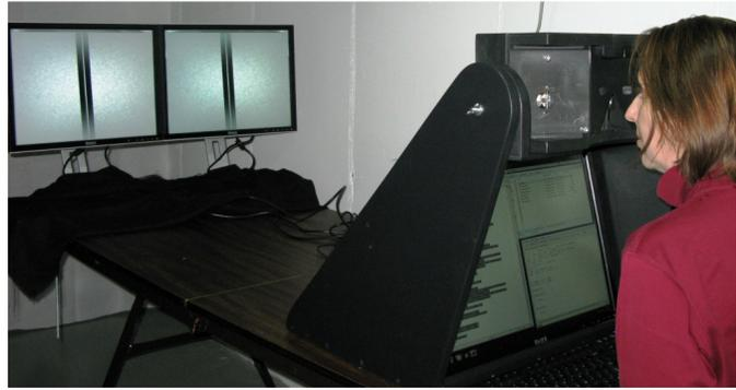
**Figure 1. Photograph of the stereoscopic display system used in the evaluation. Observers viewed a pair of LCD monitors through an optical system that set the accommodation and vergence distances to 20 m.**
