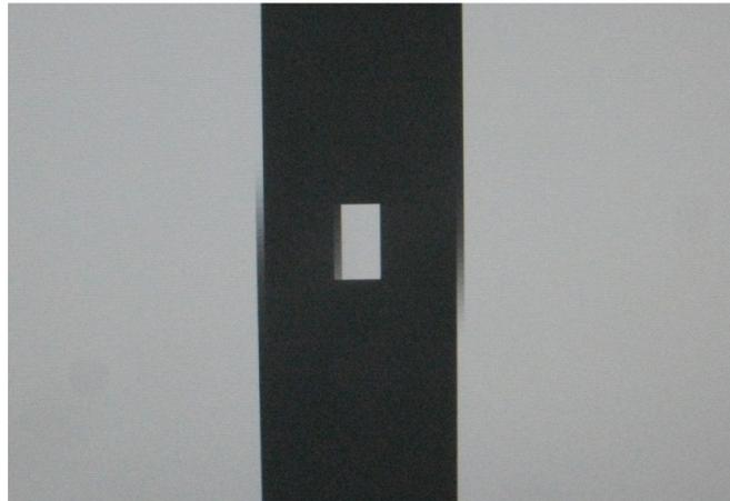
**Figure 6. Photograph of the rectangle and edge pattern showing spatial sampling artifacts. For this photograph the pixel pitch was set to 3 arcmin and the AA filter width was set to 0.7 pixels.**
