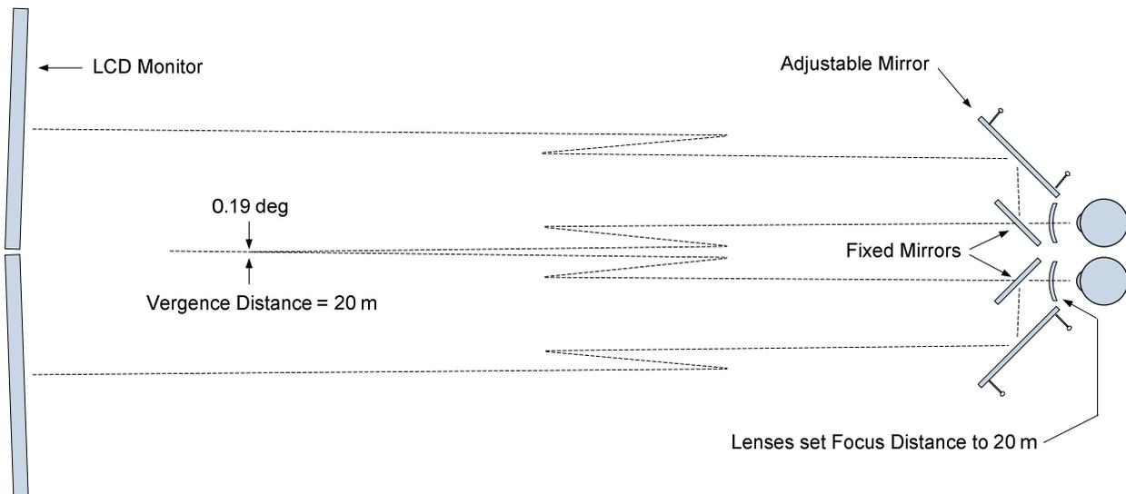
**Figure 2. Diagram of the optical layout of the display system. The outboard pair of mirrors are mounted on 3 point mounts used to set vergence distance to 20 m. The +0.5 diopter lenses extend 1.82 m display distance to a focus distance of 20 m.**
