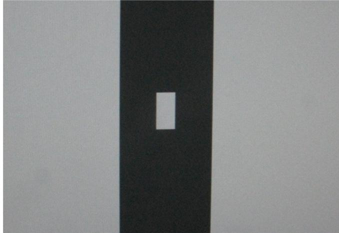
**Figure 5. Photograph of the rectangle and edge pattern used in the evaluation. The rectangle subtended an angle of 0.25 x 0.5 deg for all experimental conditions. For this photograph the pixel pitch was set to 0.5 arcmin and the AA filter width was set to 1.5 pixels.**
