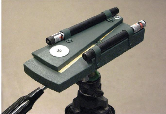
**Figure 3. Photograph of the laser vergence gauge used to calibrate and check the binocular vergence distance of the display system.**
