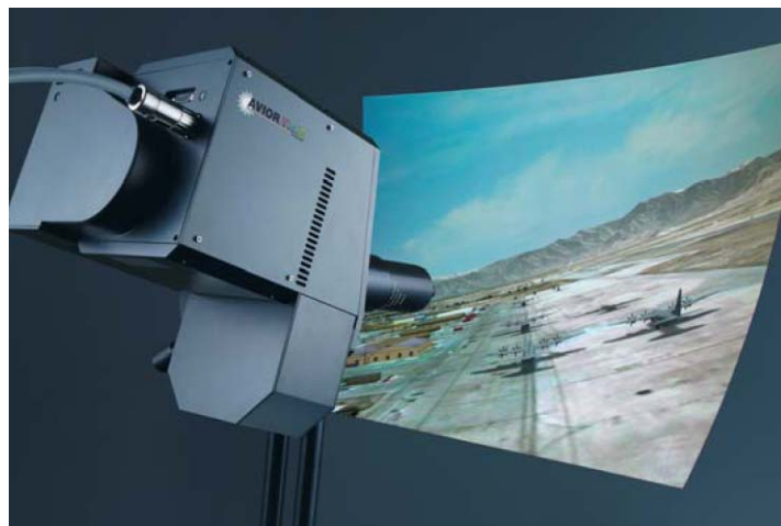
Figure 2 AVIOR ® VisIR projection head writes an image generated with VITAL X image generator.
