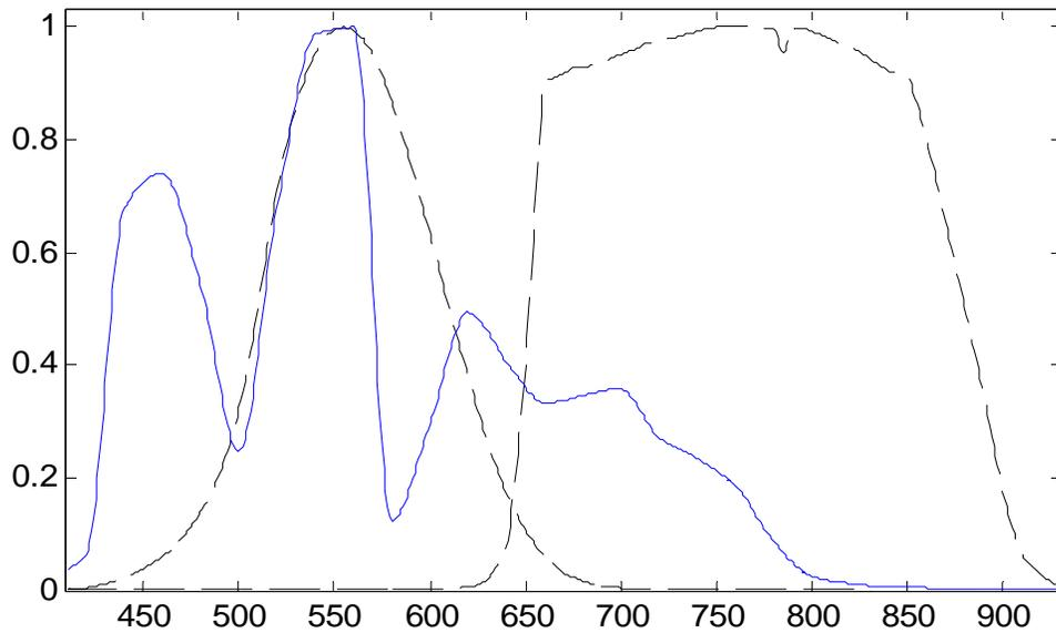
**Figure 6 Spectral power distribution of the projector with the test pattern set to full WHITE. The  $NR_v/Lum$  ratio computed from this spectra is  $0.28e-6$  W/(cm<sup>2</sup> SR fL).**
