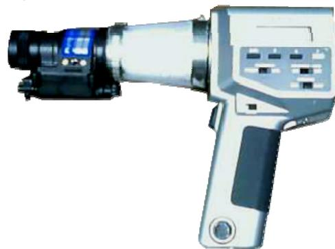
**Figure 3 Photograph of the NVG meter used at FlightSafety. Device consists of an NVG monocular attached to a Minolta LS-100 photometer with a coupling tube. This meter was calibrated against a PR-1530AR radiometer.**
