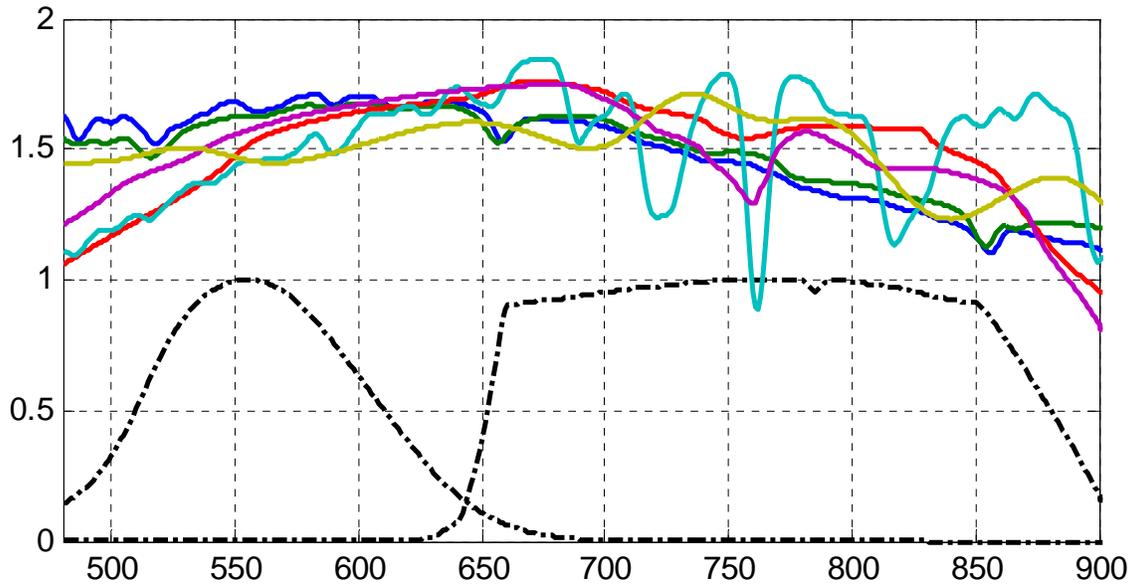
Figure 1 Upper curves: Six measurements of the spectral power distribution of lunar radiation made from the earth. The sources of these data are listed in Table 1. Lower curves: Photopic (left) and NVIS-B (right) response profiles, provided for comparison with the measured data.
