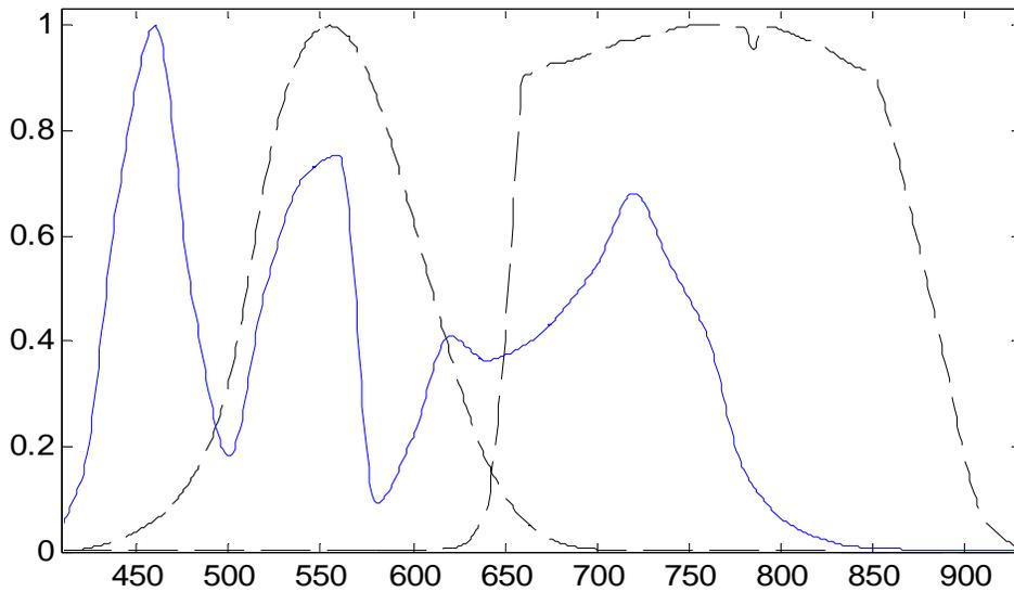
**Figure 7 Spectral power distribution of the projector with the test pattern set to BLACK. The  $NR_v/Lum$  ratio computed from this spectra is  $0.65e-6$  W/(cm<sup>2</sup> SR fL).**
