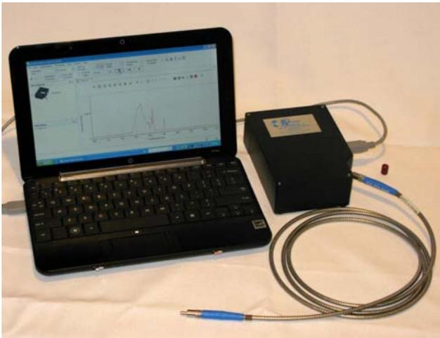
**Figure 5 Photograph of an OceanOptics HR2000+ spectrometer operated (and powered) from an HP Mini 1000 netbook computer. Light is directed into the spectrometer using the fiber optic cable (silver coil with blue ends) that would be fitted with a lens/diffuser assembly (not shown) selected for each type of measurement. Computer is running the SpectraSuite software purchased with the spectrometer.**
