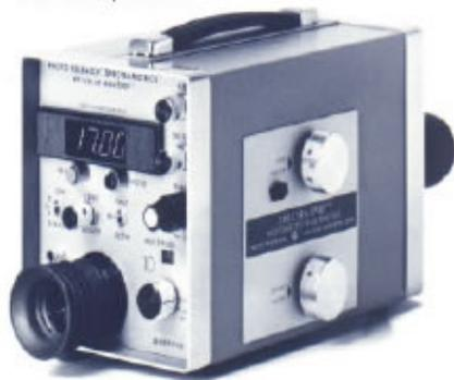
**Figure 4 Photograph of the PR-1530AR NviSpot, Night Vision Radiometer, available from Photo Research. This photomultiplier-based instrument comes with an internal calibration source and a variety of lens options that allow more flexibility in the measurement configurations.**
