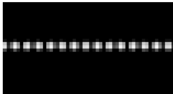
Figure 7. Sample of the horizontal line of raster lightpoints at 5 arcmin spacing as per the JAA “lightpoint size” test.
